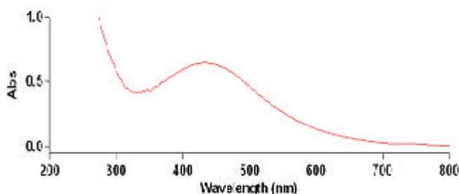
**Figure 2.** UV absorption spectra of silver nanoparticles
