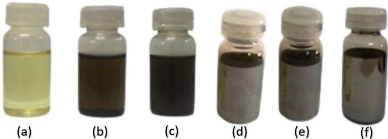
Figure 2. Visual observation of stored biopesticide (a) nutmeg seed oil (b) 1 (c) 3 (d) 5 (e) 7 and (f) 9 days
